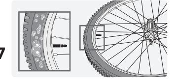
Lay tire on side and apply a thin sheen of soapy water around the sidewall and the bead area. Look for suds occurring anywhere on the tire or bead area. Suds bubbling out from the tire indicate porous areas. Shake the sealant to those areas to seal them and apply soap and water again. Check for suds forming on both sides of the tire. Repeat until no suds remain. Install the cassette and rotors according to the component manufacturer's recommendations.
