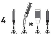
Add sealant: Once successful with inflation remove the valve core to add Stan's sealant. Add 2–3 oz. of sealant.
