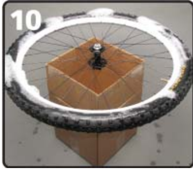
Photo 10: Lay tire parallel to the ground.
