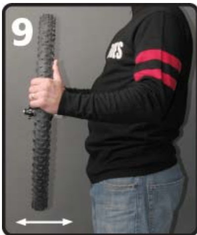
Photo 9: Bounce and rotate wheel on a hard floor to coat inside of the tire with sealant.
