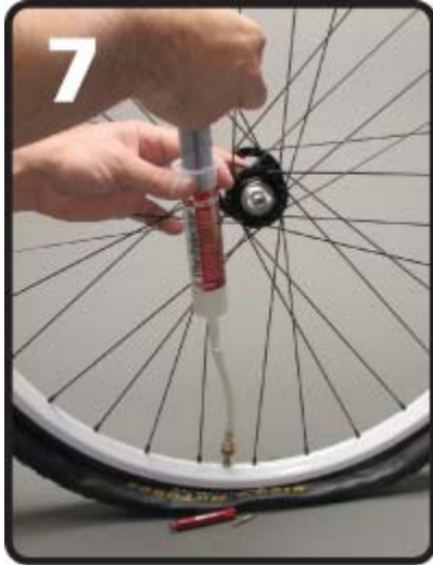
Photo 7. Adding sealant with optional injector.
