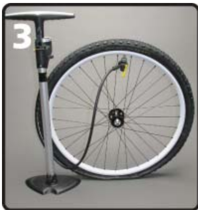
Photo 3: Hang the tire with the valve stem at the top.
