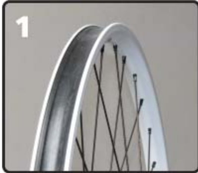
Photo 1: Correctly installed rim strip. Note: Rim strip should contact the sides of the rim and be evenly stretched.
