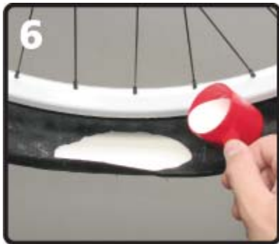
Photo 6: Adding sealant to tire using the scoop provided.
