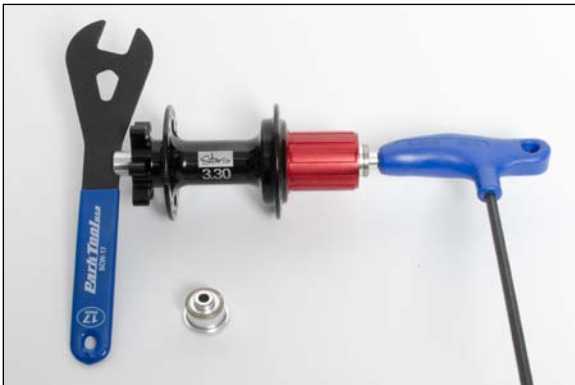
Figure 1 Type II – Drive side end cap removal
