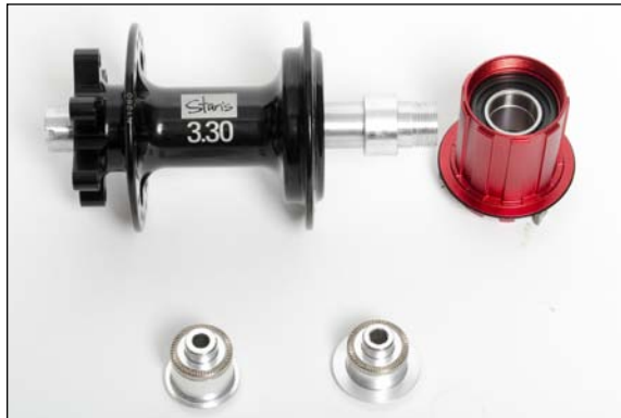
Figure 2 Type II – End caps removed
