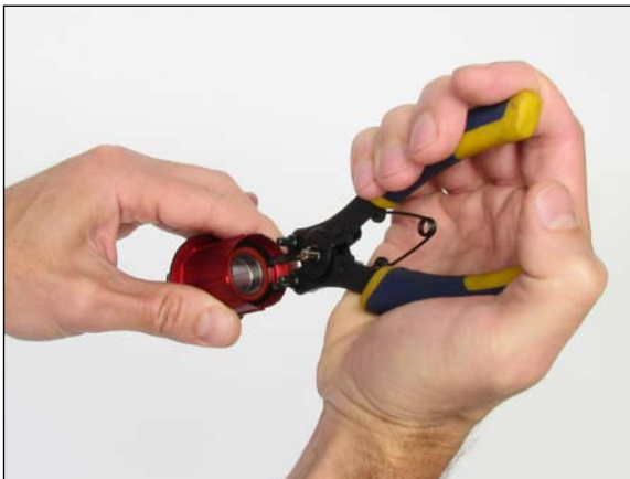
Figure 10 – Retaining ring removal
