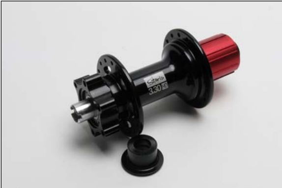
Figure 6 – End cap removed non-drive side
