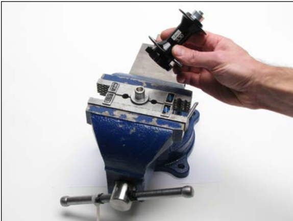
Figure 14 – End Cap removal
