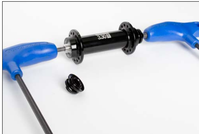
Figure 19 - 2nd End cap removal
