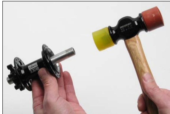
Figure 2 – Bearing removal non drive side
