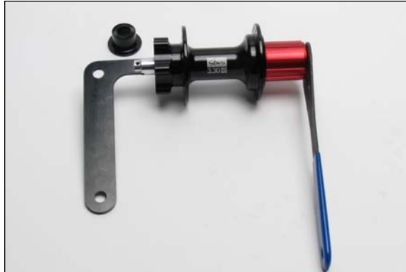
Figure 7 – End cap removal drive side
