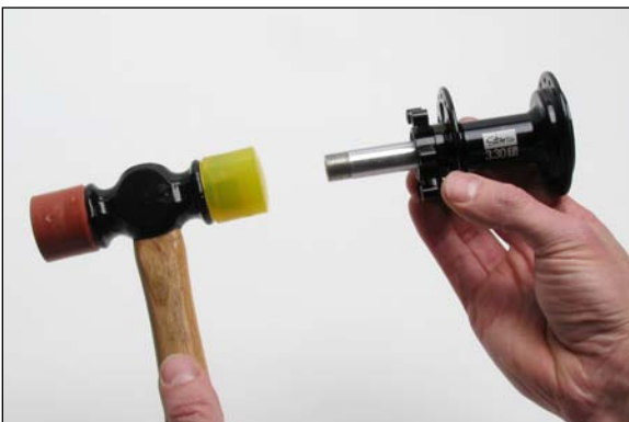
Figure 3 - Bearing removal drive side
