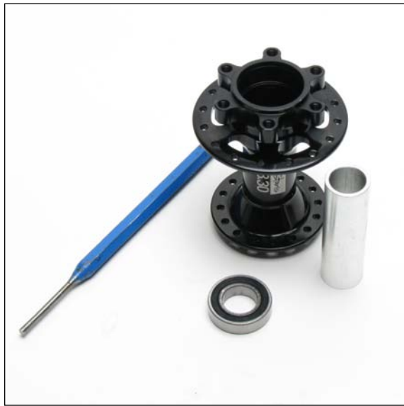
Figure 17 - Bearing and sleeve removed
