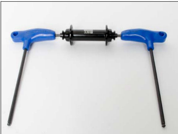
Figure 18 - 1st End cap removal
