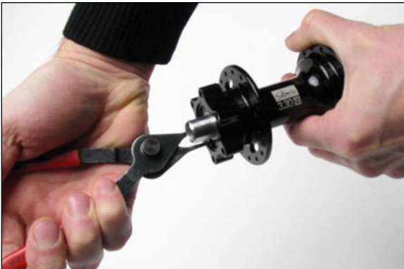
Figure 8 – Retaining ring removal
