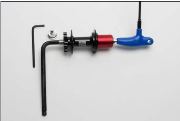
Figure 1 – End cap removal
