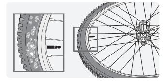
Lay tire on side and apply a thin sheen of soapy water around the sidewall and the bead area. Look for suds occurring anywhere on the tire or bead area. Suds bubbling out from the tire indicate porous areas. Shake the sealant to those areas to seal them and apply soap and water again. Check for suds forming on both sides of the tire. Repeat until no suds remain. Install the cassette and rotors according to the component manufacturer's recommendations.
