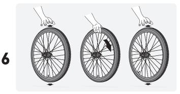
Bounce: hold the wheel vertically and gently bounce or "dribble" it to disperse the sealant throughout the inside of the tire. Let it drop from an inch or two, then rotate a few degrees and repeat. Do this for several revolutions of the wheel.
