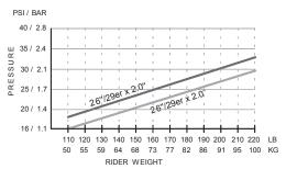
Inflate to riding pressure; the chart above is a recommended starting point. Always review the maximum pressure information listed on both the rim and the tire and consider the lower of the two numbers your maximum pressure. Do not inflate above the lower of the two numbers.
