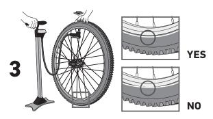
Rotate the valve to 12 o'clock and install a pump. Inflate tire to 35psi to seat tire.
