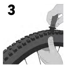
Align tip of DART tool with puncture and push tip and DART material into the puncture until the body of the DART tool contacts the tire and the barbs are completely inserted into the tire.
