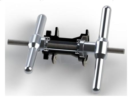
7. Turn the handle clockwise to press the bearing into the hub until it is hand-tight and the bearing is fully seated in the hub shell. (*Note: Over-tightening can result in bearing damage.*)
