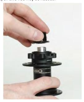
• Remove axle and drive-side endcap by hand. If the axle will not remove by hand, tap on the exposed (non-drive) axle end with a soft-face hammer to dislodge.
