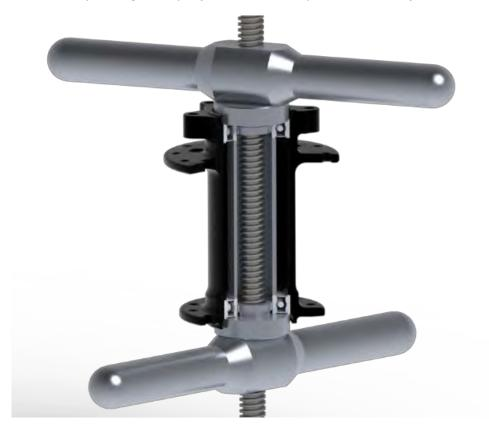
8. Turn the handle clockwise to press the bearing into the hub until it is hand-tight and the bearing is fully seated in the hub shell (*Note: overtightening can result in bearing damage*).
