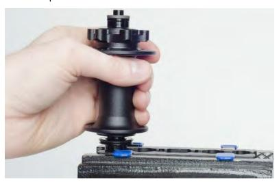
• For **15mm** End cap: Clamp one end cap in the **20mm** slot of the Park Tool AV-5. Gently rock the hub/wheel toward you to unseat the cap. Repeat on the other end cap.
