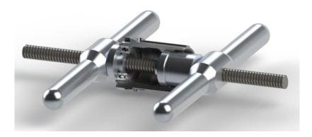
3. Arrange the freehub body, bearing press, 15267 open bore drifts, and one 15267 bearing as shown below. (*Note: Installing one bearing at a time ensures the bearing is installed straight*).
