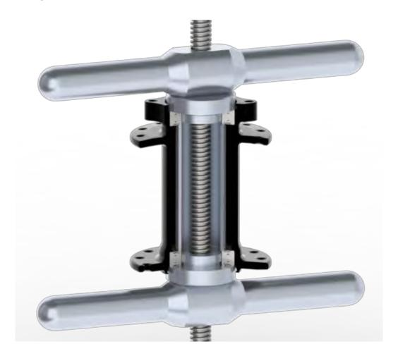
8. Turn the handle clockwise to press the bearing into the hub until it is hand-tight and the bearing is fully seated in the hub shell (*Note: overtightening can result in bearing damage*).
