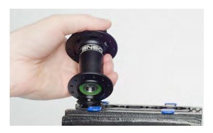
Clean end caps before reinserting into the hub. (Note: Cleansing of the end cap seals should be performed in accordance with Section 1.5 to prevent damaging them). Ensure that the SealLock seals are positioned with their U-hook facing outwards from the hub body, as shown below. Install end caps, taking care to not pinch or fold the SealLock seal
