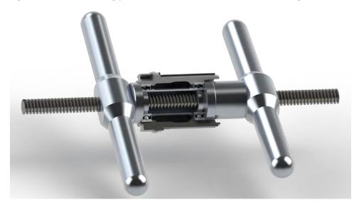
8. Turn the handle counter-clockwise to press the bearing into the hub until it is hand-tight and the bearing is fully seated in the hub shell. (*Note: Over-tightening can result in bearing damage.*)
