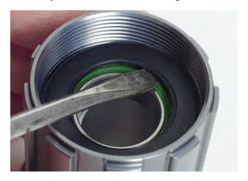
3. Insert 15mm Sealed Bearing Extractor into one of the freehub bearings. Tap Extractor and bearing out of hub shell using punch and hammer, as shown in the following image. (Note: Perform this step over a rag as the bearing, extractor, and inner axle sleeve will fall from the hub shell when the bearing is removed.)
