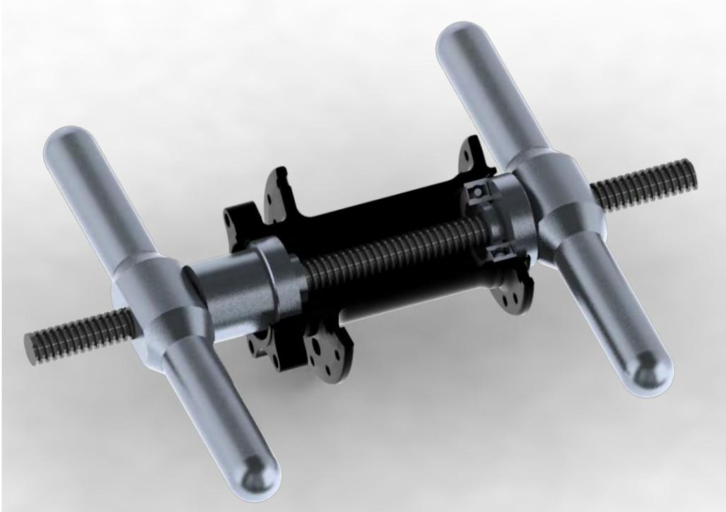
4. Turn the handle clockwise to press the bearing into the hub until it is hand-tight and the bearing is fully seated in the hub shell (*Note: Overtightening can result in bearing damage*).
