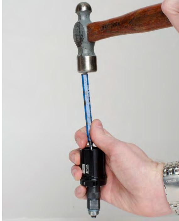
4. Install 15mm Sealed Bearing Extractor in the second bearing. Tap Extractor and bearing out of hub shell using punch and hammer.
