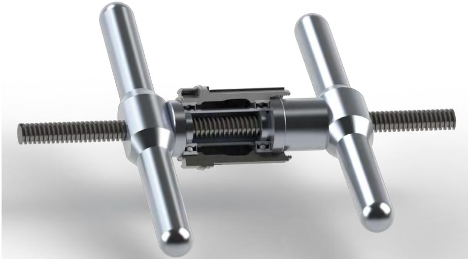
8. Turn the handle counter-clockwise to press the bearing into the hub until it is hand-tight and the bearing is fully seated in the hub shell. (*Note: Over-tightening can result in bearing damage.*)
