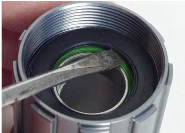
3. Insert 15mm Sealed Bearing Extractor into one of the freehub bearings. Tap Extractor and bearing out of hub shell using punch and hammer, as shown in the following image. *(Note: Perform this step over a rag as the bearing, extractor, and inner axle sleeve will fall from the hub shell when the bearing is removed.)*
