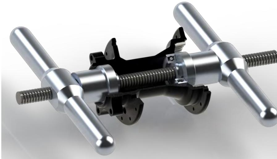
4. Turn the handle clockwise to press the bearing into the hub until it is hand-tight and the bearing is fully seated in the hub shell. Note: Over-tightening can result in bearing damage.
