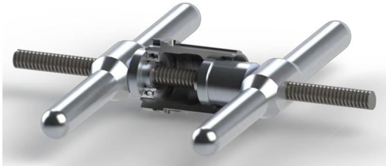
3. Arrange the freehub body, bearing press, 15267 open bore drifts, and one 15267 bearing as shown below. *(Note: Installing one bearing at a time ensures the bearing is installed straight).*
