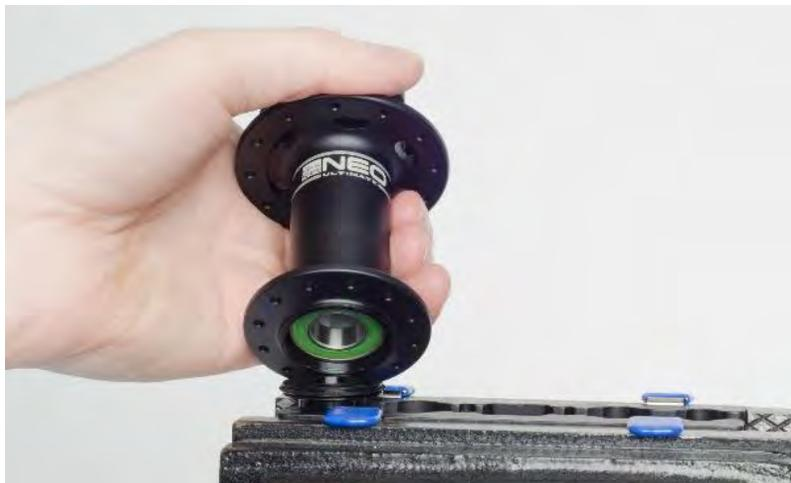
2. Clean end caps before reinserting into the hub. (*Note: Cleansing of the end cap seals should be performed in accordance with Section 1.5 to prevent damaging them*). Ensure that the SealLock seals are positioned with their U-hook facing outwards from the hub body, as shown below. Install end caps, taking care to not pinch or fold the SealLock seal
