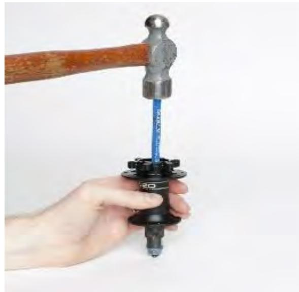
3. Remove the inner axle sleeve.
